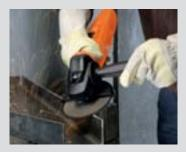
Easily remove burrs from the edges of roughly machined work pieces without residue.
